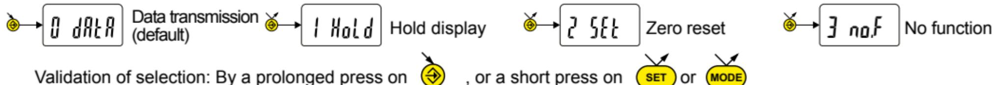
**Note:** a function can also be assigned via RS232 using the command <FCT + Function No.> (FCT 0...3)
