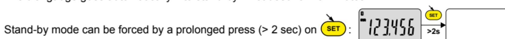
In stand-by mode, the value of the origin is retained by the sensor (SIS mode), and the instrument automatically restarts with any movement of the measurement probe, RS command or press a button.
